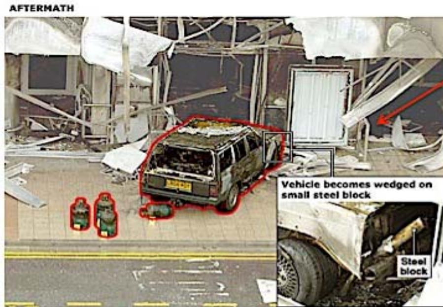
Figure 16. Glasgow Airport Attack on Main Terminal. 368
